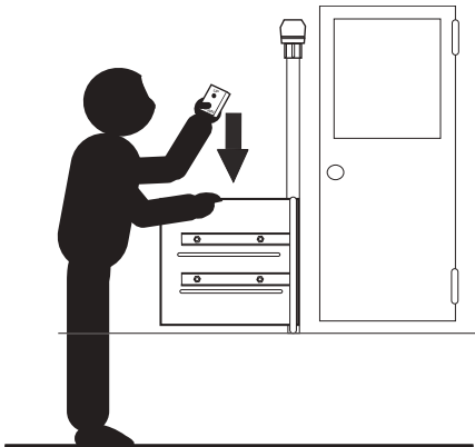
1. Remove Safety pin and lower plate.
