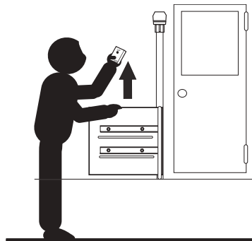
5. Raise platform till it latches securely.
