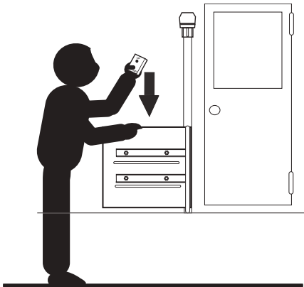
1. Remove Safety pin and lower plate.
