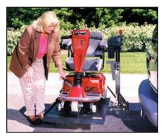
Once your scooter is on the platform and the brake is locked, push the switch to raise and stop halfway. Attach the adjustable safety belts. Finish raising until the Mobile-Lift automatically locks into place. Then just drive away!
