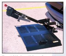
The unit folds down 45 degrees for access to the car's trunk, or the rear of station wagons, vans, or pick-up trucks.
