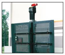
The Mobile-Lift Outside Model folds up out of the way when not in use. Just unfasten the lockup strap and lower platform when ready to use.
